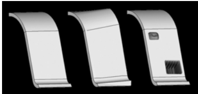
figure 4: Concept-1, extending the technology of the Continuum Robot to create three types of morphing surfaces: bending, twisting, and shape-shifting [authors].
