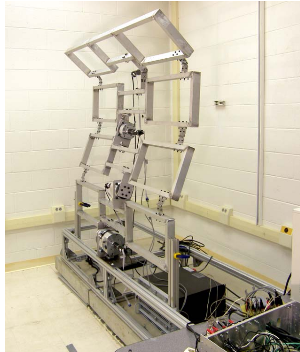
Figure 2. Developing prototype of the robotic “wall” showing four of its eight panels.
