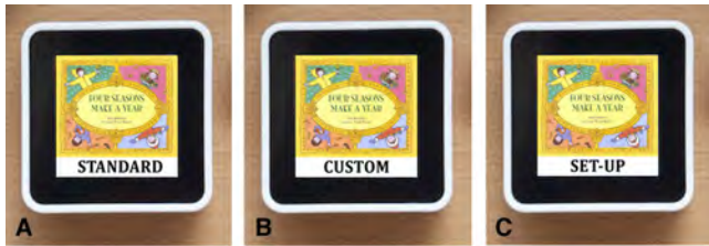
Figure 14. A: Sifteo™ standard option screen. B: Sifteo™ custom option screen. C: Sifteo™ custom set-up screen.
