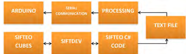
Figure 12. Sifteo™ / Arduino communication diagram.
