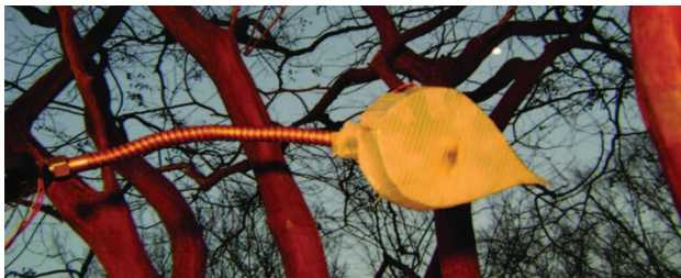
Figure 4. Project 2—The Directing Leaf: the leaf was designed to work with existing urban infrastructure in the event of tornadoes around or within city limits. In the event of a tornado sighting, the leaf would light up and point the population toward shelters and safer areas. A radio link to a receiver and speaker system would play area-specific warning messages to complement the visual aids. Upon relaxation of the situation, the leaves would return to their resting state and the speaker system would update the population. This system was designed to blend into the environment, though not inconspicuously, and was also capable of lighting up street blocks during festive seasons.
