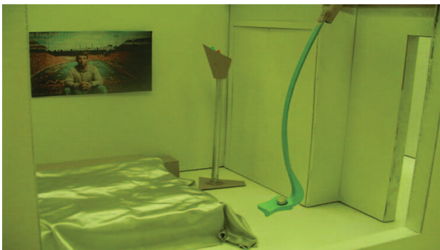
Figure 8. Project 3—The Emotionally Together Armature (ET): ET consists of an overhead two-degree-of-freedom robot crane capable of motion along the length and width axes of a single room. A hanging armature picks up and deposits objects while using infrared sensors to avoid obstacles. ET was proposed with an option to minimize aspects of loneliness by analyzing the occupant's voice for emotional affect and then providing an automated response.
