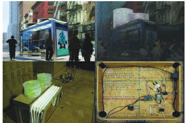
Figure 6. Project 2—The Particulate Control and Air Purifier (pCAP): added onto existing city infrastructure, pCAP was designed as an urban response mechanism to minimize the dispersion of airborne particulates and gases while providing shelter and purified air to those trapped within the noxious atmosphere. Augmented bus shelters would function as glowing beacons in the dusty haze, where purified air would be available. The pCAP used modified fire suppression sprinkler heads mounted on building parapets and actuated by gas and vibration sensors to produce atmospheric mist to trap the particulates.
